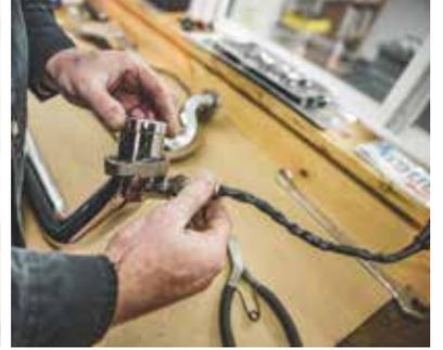
2. A) Remove retaining rings & flanges from stock exhaust.
