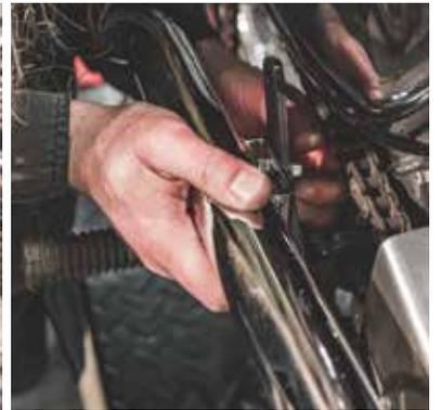
4. Loosely install pipes on cylinder heads & rear bracket.
