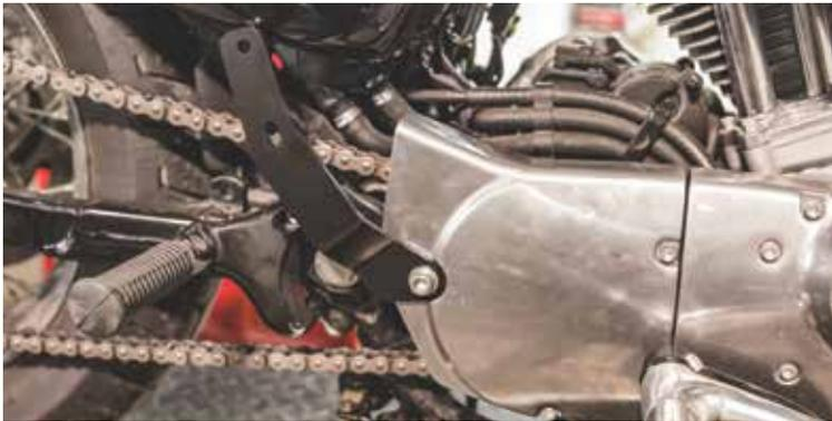
3. Re-install pulley cover & install bracket from kit.
